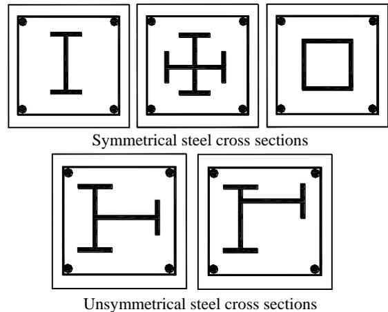
Fig. 1 Types of concrete-encased steel composite column
