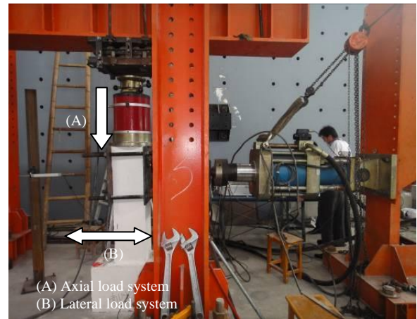
Fig. 3 Test set-up for cyclic loading test
