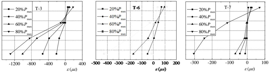
Fig. 8 Strain distributions of concrete along cross-section.
