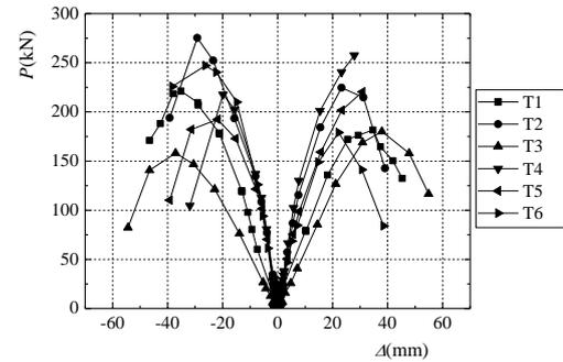
(a) T-shaped steel section specimens ( $\lambda=2.5$ )
