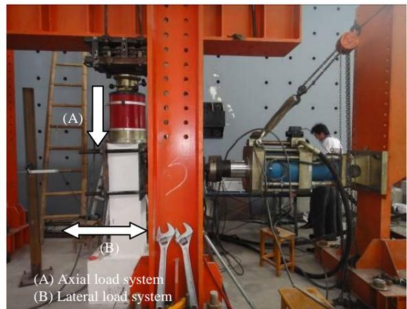
**Fig. 3** Test set-up for cyclic loading test
