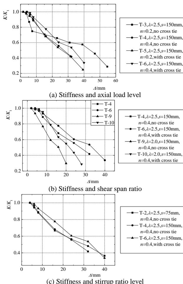
Fig. 13 Relationships between the stiffness and displacement
