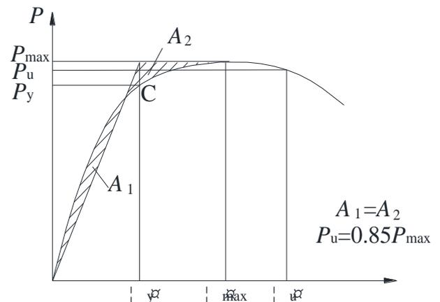
**Fig. 12** Definitions of yield point and failure point
