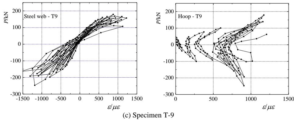
Fig. 9 Strain distribution of steel web and hoop
