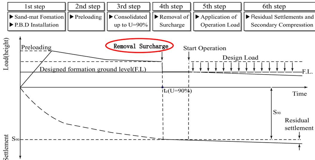
Fig. 1 Flow of ground improvement with PBDs
