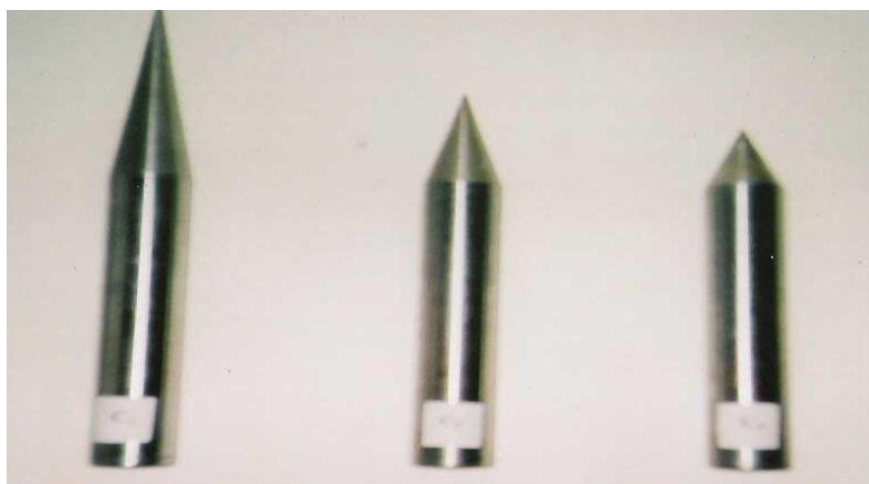
Fig. 1 Ogival nose projectiles with nose angles of 15°, 30° and 45°
