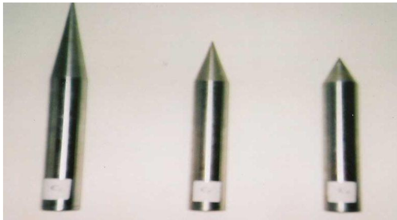
Fig. 1 Ogival nose projectiles with nose angles of 15^\circ , 30^\circ and 45^\circ
