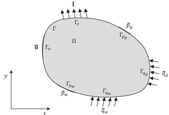
Fig. 1 Boundary conditions of the body  $\Omega$
