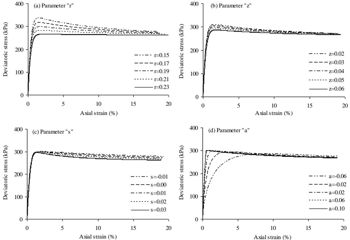
**Fig. 3** Sensitivity analysis for deviatoric stress-axial strain curves ( $p_0=100$  kPa,  $Dr=70\%$ ,  $GC=29.33\%$ ) (a) Parameter  $r$  (b) Parameter  $z$  (c) Parameter  $s$  (d) Parameter  $a$
