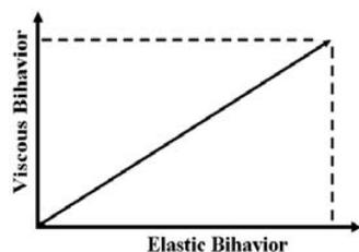
Fig. 1 Components of total complex shear modulus.
