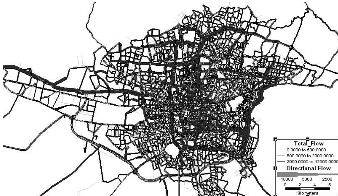
Fig. 2 Traffic volumes obtained from the CTDAM during a peak hour for Tehran network in 2007.
