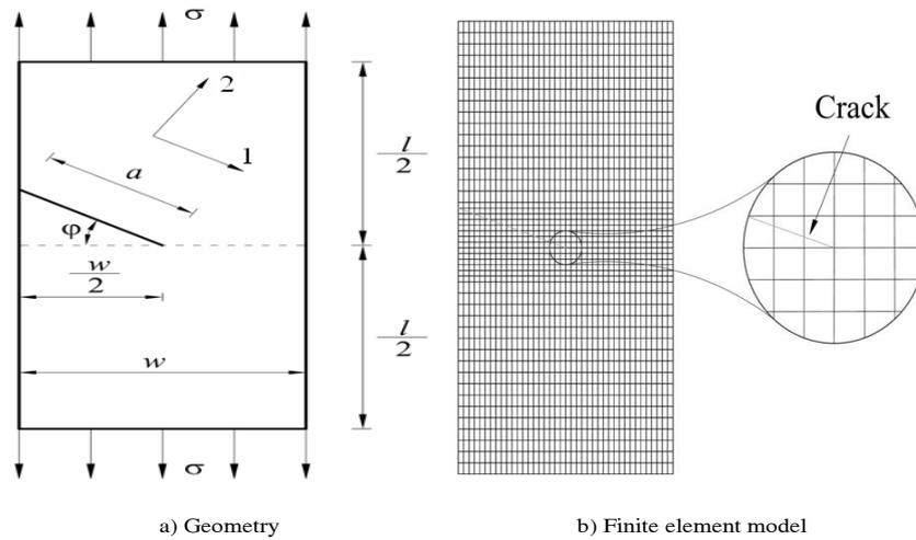
**Fig. 10** Specimen geometry of a rectangular plate with single notched cracked.
