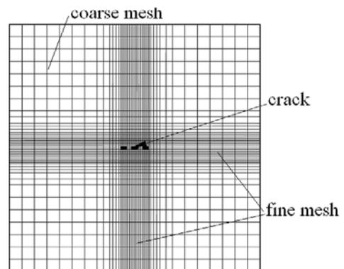
**Fig. 9** The discretized adaptive finite element model.
