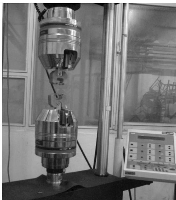
Fig. 5 Experimental setup for BRB tests
