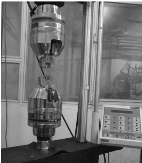
Fig. 5 Experimental setup for BRB tests
