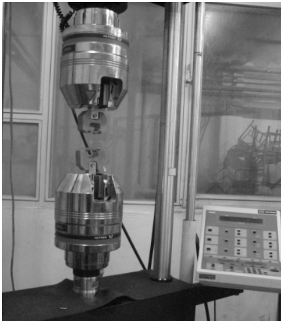
Fig. 5 Experimental setup for BRB tests
