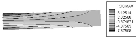
**Figure 7** Contours of  $\sigma_x$  stress (Regular grid of 1649 nodes)
