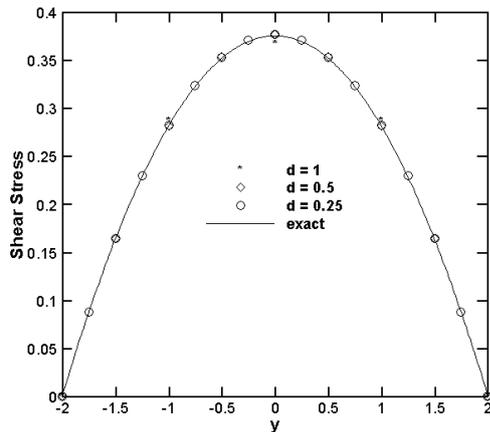
**Figure 5** The shear stress distribution of cantilever beam at  $x=L/2$
