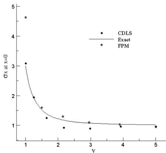
**Figure 17** The normal stress  $\sigma_x$  along  $x = 0$
