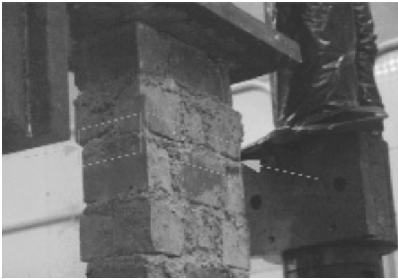
Fig. 8 Failure development in masonry sample No.3 at last loading step
