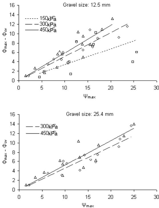
**Fig.10** Bolton's [8] equation for sand-gravel mixtures tested under different surcharge pressures
