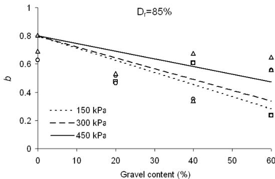
**Fig.11** Variation of b coefficient with minimum void ratio for different surcharge pressures
