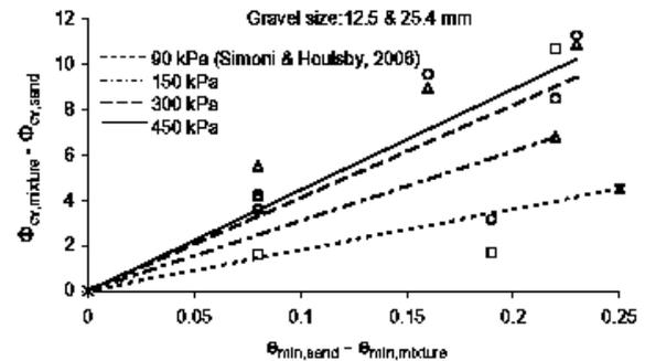
**Fig.14** Empirical equation describing the variation of constant volume friction angle of different mixtures with minimum void ratio
