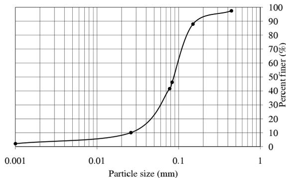
Fig. 1a Particle size distribution of fly ash
