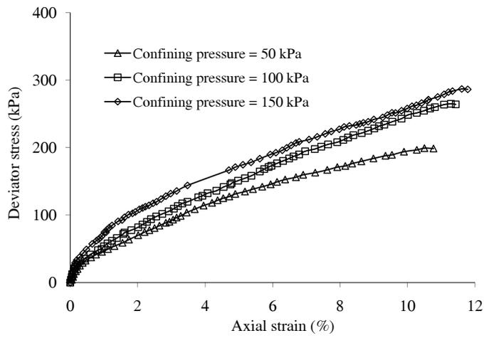
**Fig. 6** Stress-strain diagram of plain soil
