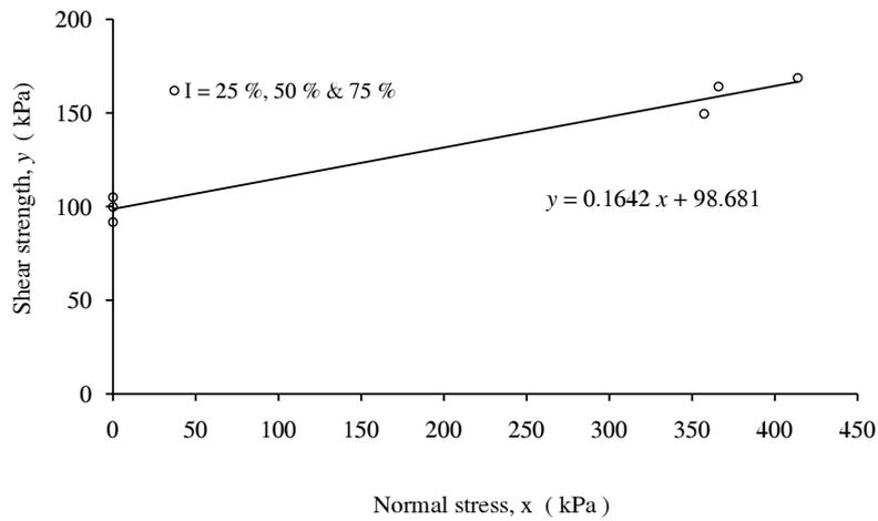
**Fig. 16** Failure envelop for soil-fly ash matrix (N=10)
