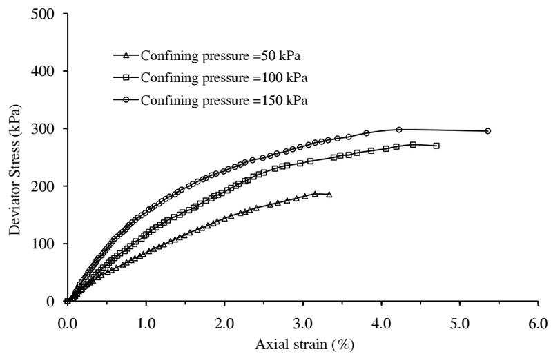
**Fig. 8** Stress-strain diagram of layered sample for N=0
