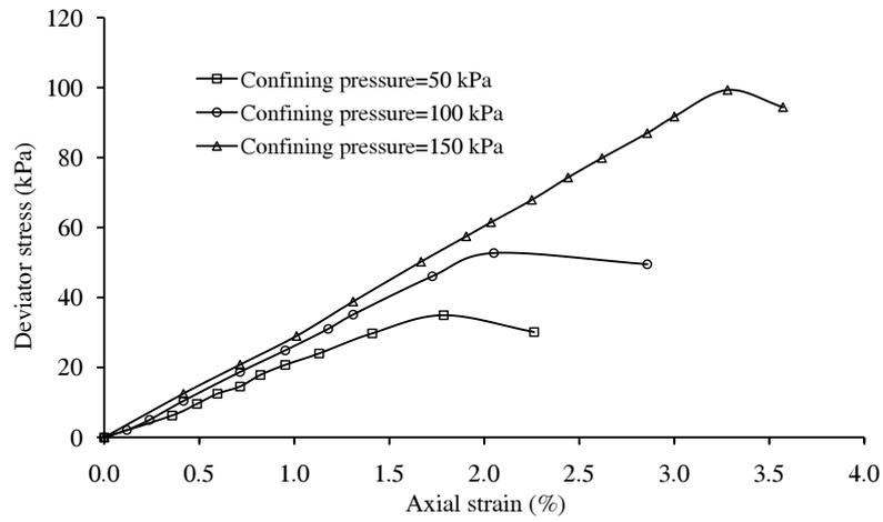
**Fig. 7** Stress-strain diagram for plain fly ash
