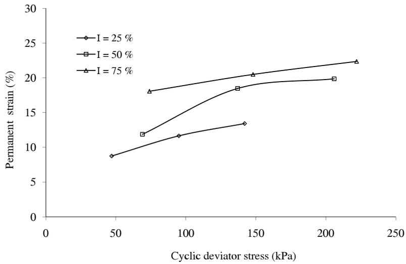
**Fig. 15** Plot showing variation of permanent strain and cyclic deviator stress
