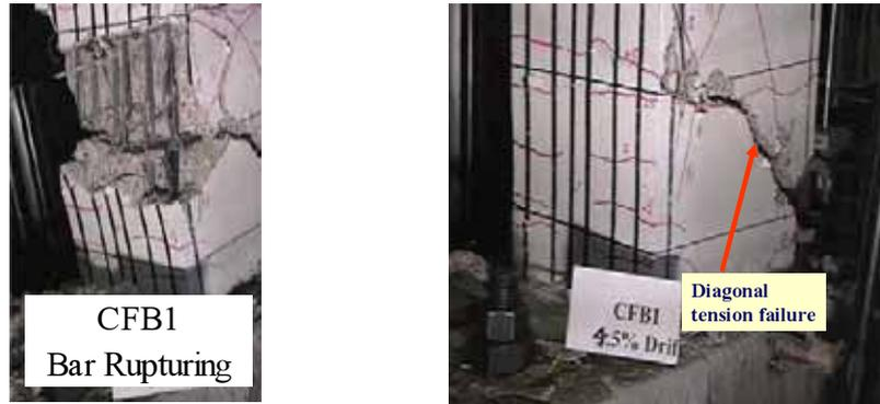
**Fig.4** Observed Damages in Beam CFB1
