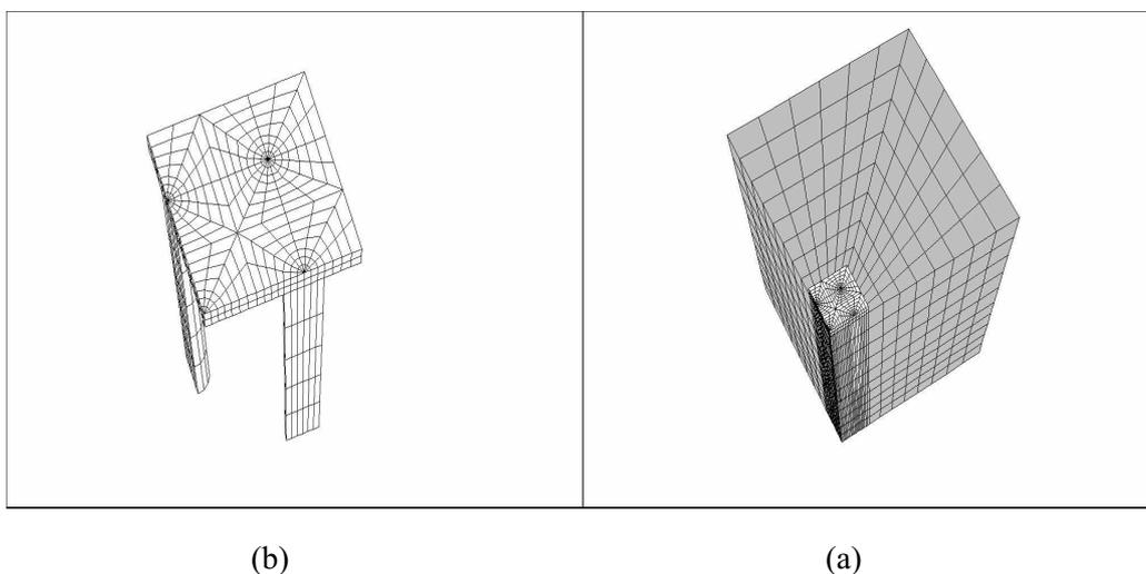
Fig. 3. Numerical model of pile-raft foundation under 1g physical test using FLAC-3D
