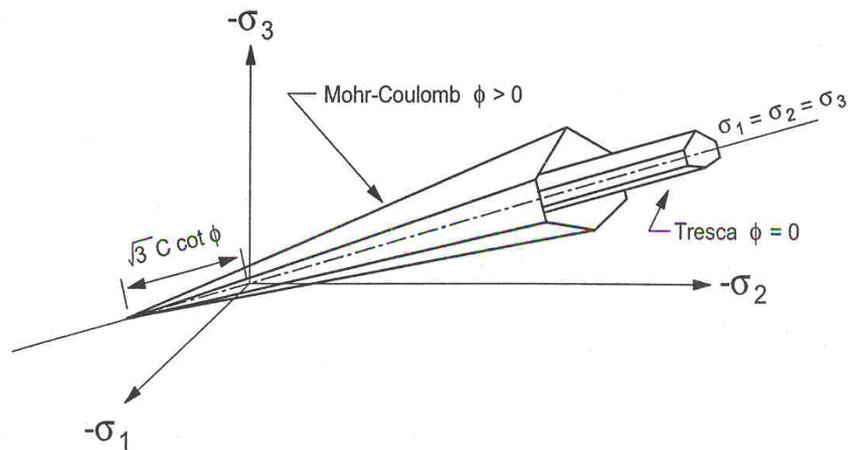
Fig. 2. Mohr – Coulomb constitutive model used in present study to model nonlinear behavior of medium dense sand
