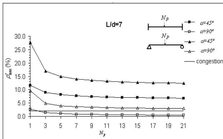
**Fig.2.** Effect of the bending to the shear loading ratio for s-s and Fixed Ended beams ( $h=800\text{mm}$ ,  $b=400\text{mm}$ ,  $f'_c=80\text{MPa}$ ,  $f_y=400\text{MPa}$ ,  $\phi = \phi' = 25\text{mm}$ ).
