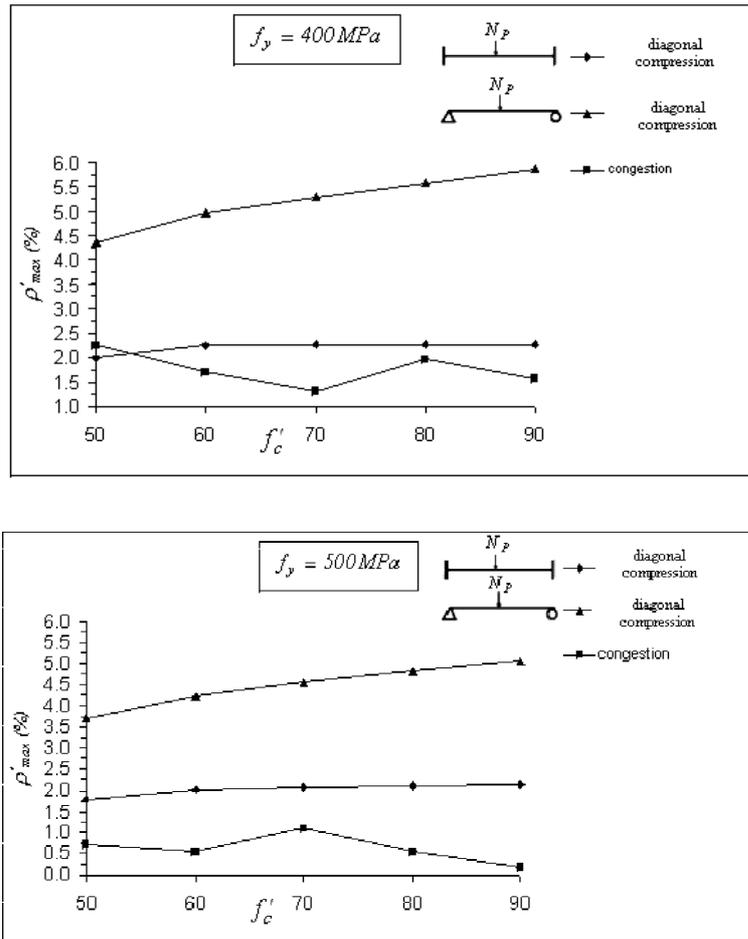
Fig.4. Effect of concrete and steel strength on  $\rho'_{max}$  for Fixed Ended beam and simply supported beam loaded with uniformly distributed load ( $h=800\text{mm}$ ,  $b=400\text{mm}$ ,  $L/d=10$ ,  $\phi = \phi'=25$ ,  $\alpha = 90^\circ$  ).
