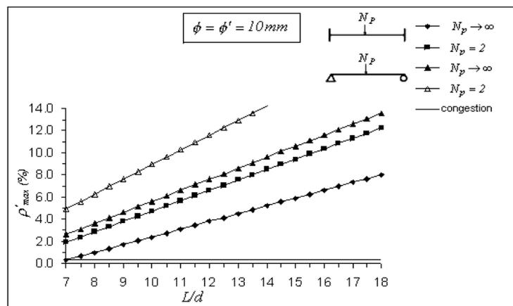
Fig.3. Effect of beam's  $L/d$  ratio on  $\rho'_{max}$  for Fixed ended beam and simply supported beam loaded with two concentrated loads and with uniformly distributed load ( $h=800mm$ ,  $b=400mm$ ,  $f'_c=80MPa$ ,  $f_y=400MPa$ ,  $\alpha=90^\circ$ ).
