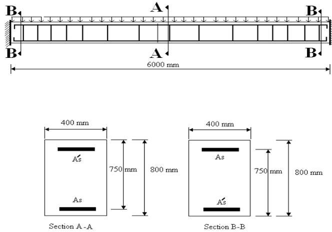
Fig.5. Beam dimensions for section A-A and B-B.
