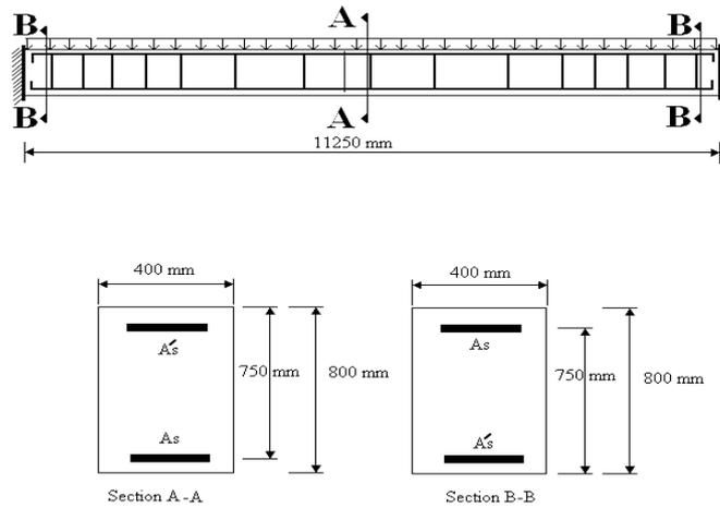
Fig.6. Beam dimensions for section A-A and B-B
