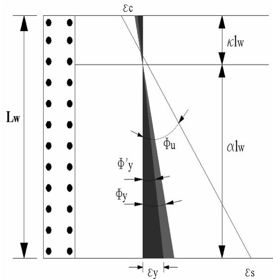
Fig.3 compressive strain and curvature of shear wall section
