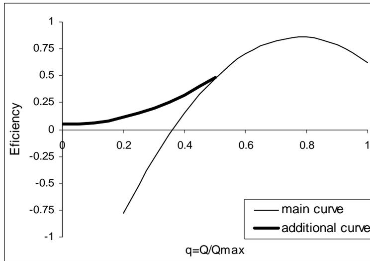
Fig. 1 Efficiency-relative discharge curves for specified pump types
