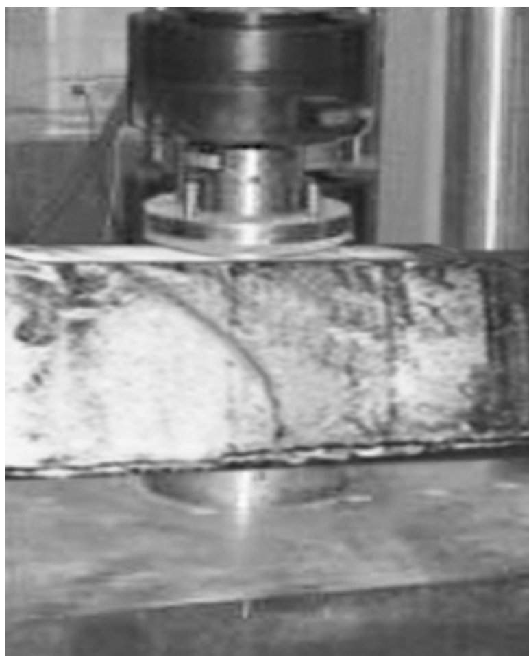
Fig. 4 Shear Failure of Beam with GFRP
