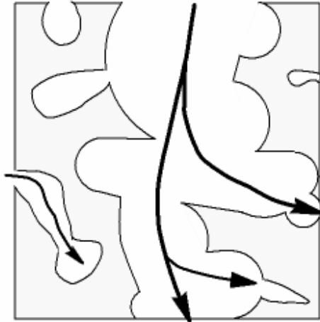
Fig.1 Flow through a typical porous specimen.
