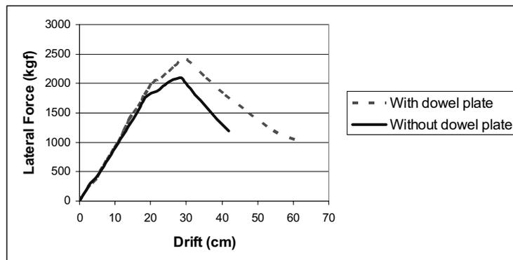
Fig.9 Effect of dowel plates on pushover diagram
