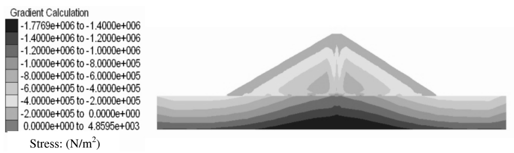
Figure 8: Vertical stress contours on dam cross-section (static analyses)
