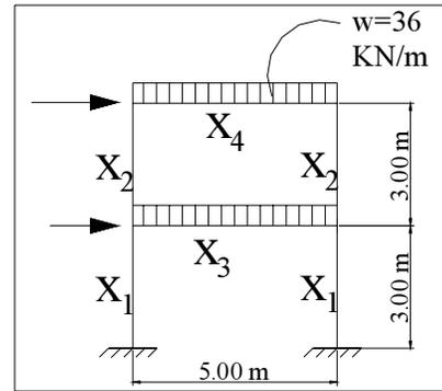
Figure 2: A two-story, one-bay frame under seismic loading.
