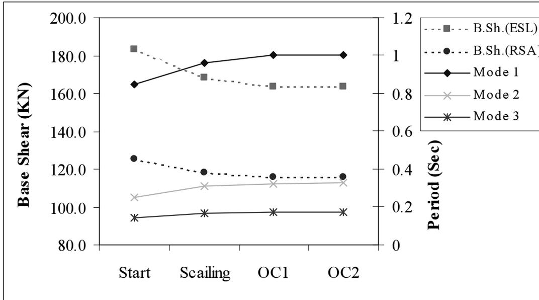
Figure 7: Variation of the first 3 natural periods and base shears (ESL and RSA methods) of the frame of Example 2.
