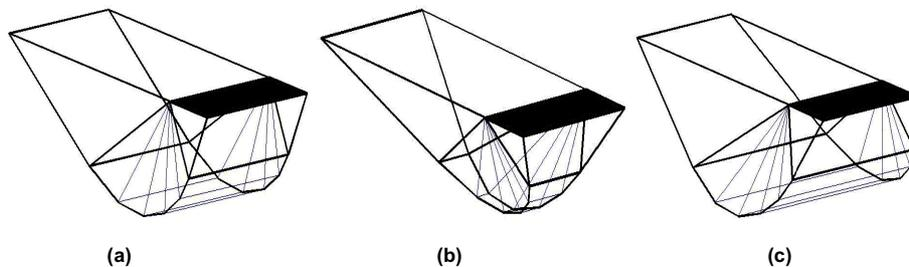
Fig. 5. The inclination of lateral failure surfaces in the three dimensional space, (a)- zero value for  $\theta_1$  and  $\theta_2$  (vertical), (b)- negative value (inclined inwards), (c)- positive value (inclined outwards).
