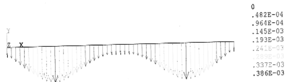
Fig. 13. Deflection factor of dynamic load case (Train speed=30 Km/h).
