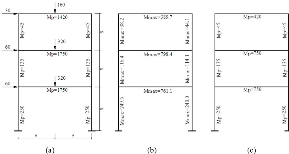
Fig. 6. 1-bay and 3-story frame (a) geometry, boundary conditions and upper bound of plastic moments (b) maximum obtained moment for each member (c) selected plastic moments in Reference [2].
