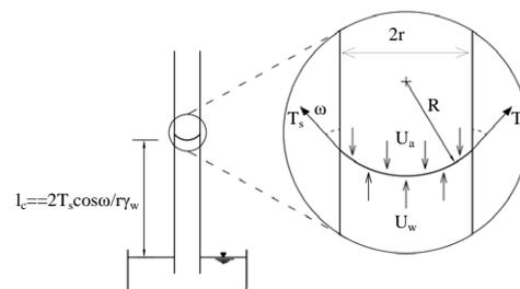
Fig. 1. The capillary rise in narrow tube and the equilibrium condition at meniscus
