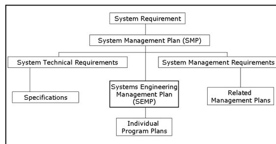
Fig. 1. Place of SEMP in system management plans
