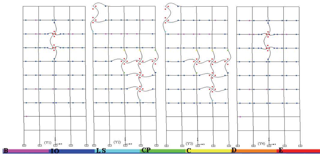
Fig. 6. Plastic hinge formation status in 10 story building under Tabas excitation with PGA=0.7g
