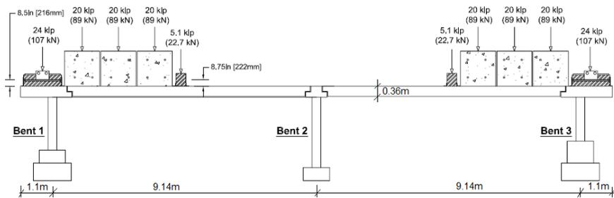
Fig. 1 Elevation and top view of two-span bridge [1]
