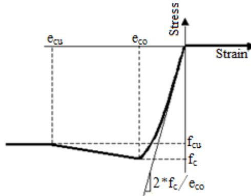
Fig. 3 Concrete01 Material Parameters [7]
