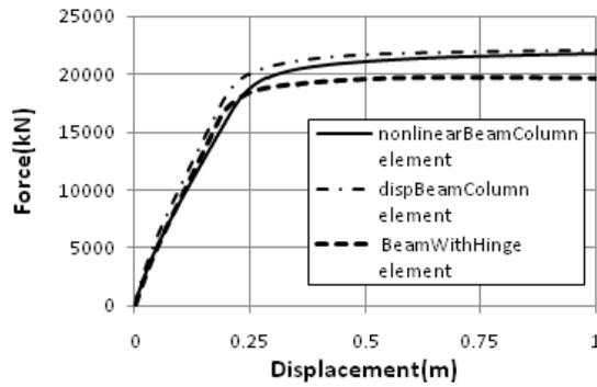
Fig. 10 Longitudinal capacity curve of east Bridge
