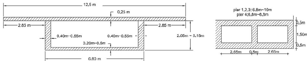
**Fig. 9** Member Cross Sections of RH Bridge
