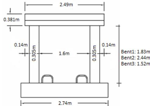
Fig. 2 two-span bridge bents [1]
