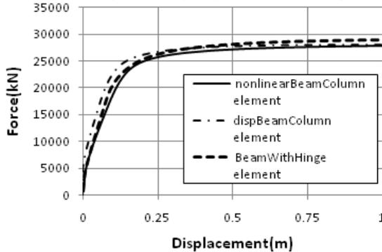
Fig. 12 Transverse capacity curve of east Bridge
