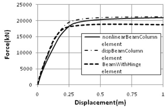
Fig. 11 Longitudinal capacity curve of west Bridge
