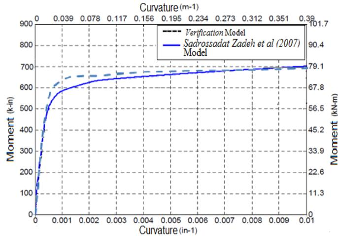
Fig. 5 Moment-Curvature curve for the Column Section of two-span Bridge
