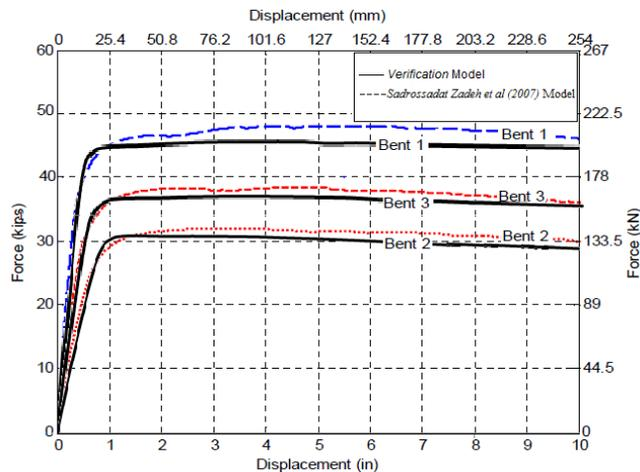
Fig. 6 Capacity curves of two-span Bridge Bents
