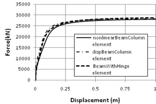
Fig. 13 Transverse capacity curve of west Bridge
