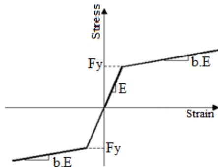
Fig. 4 Steel01 Material Parameters [1]
