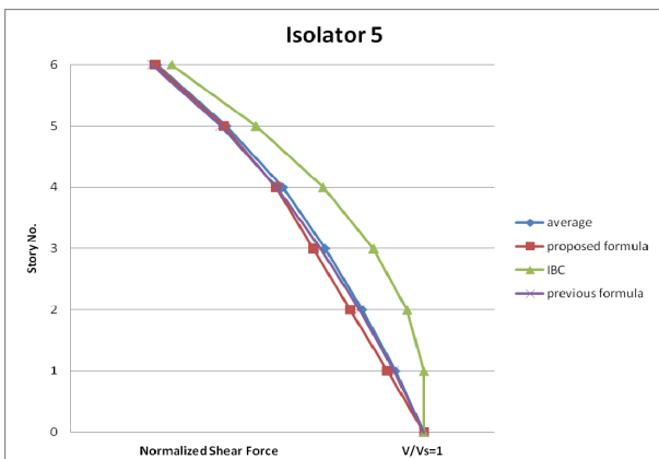
Fig. 14 Comparison of nonlinear dynamic analysis, IBC formula, proposed formula in section 6 and previous formula for 6 story building
