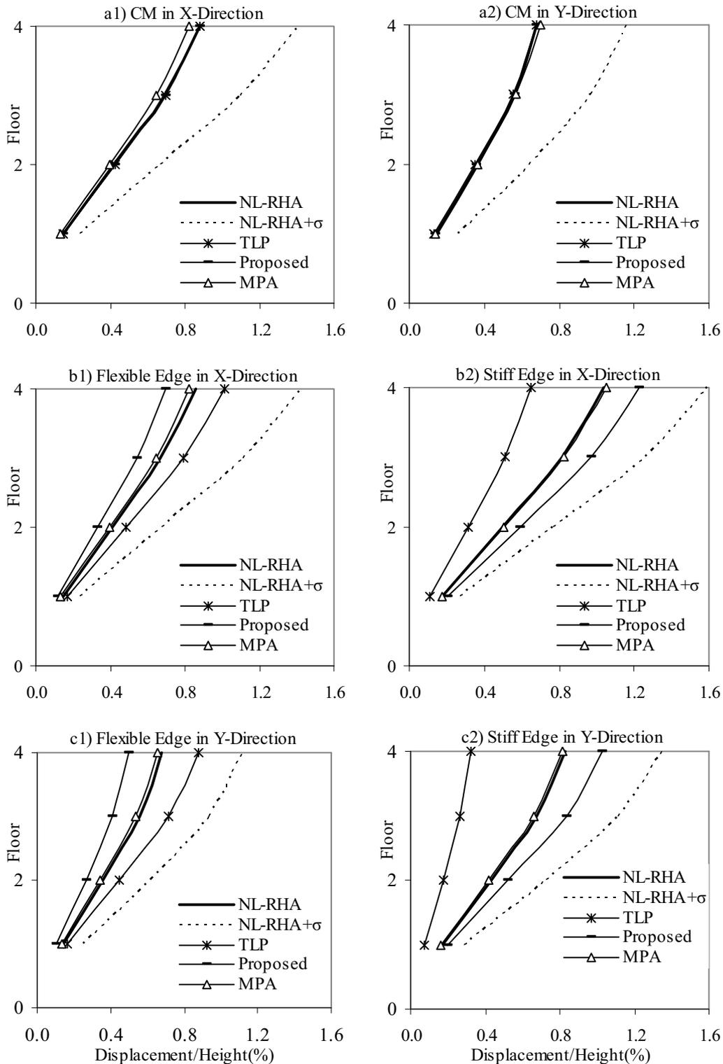
**Fig. 6** Height-wise variation of the displacements for the torsionally-flexible 4-storey building: a) at the CM; b) at the flexible and stiff edges in X-direction; and c) at the flexible and stiff edges in Y-direction
