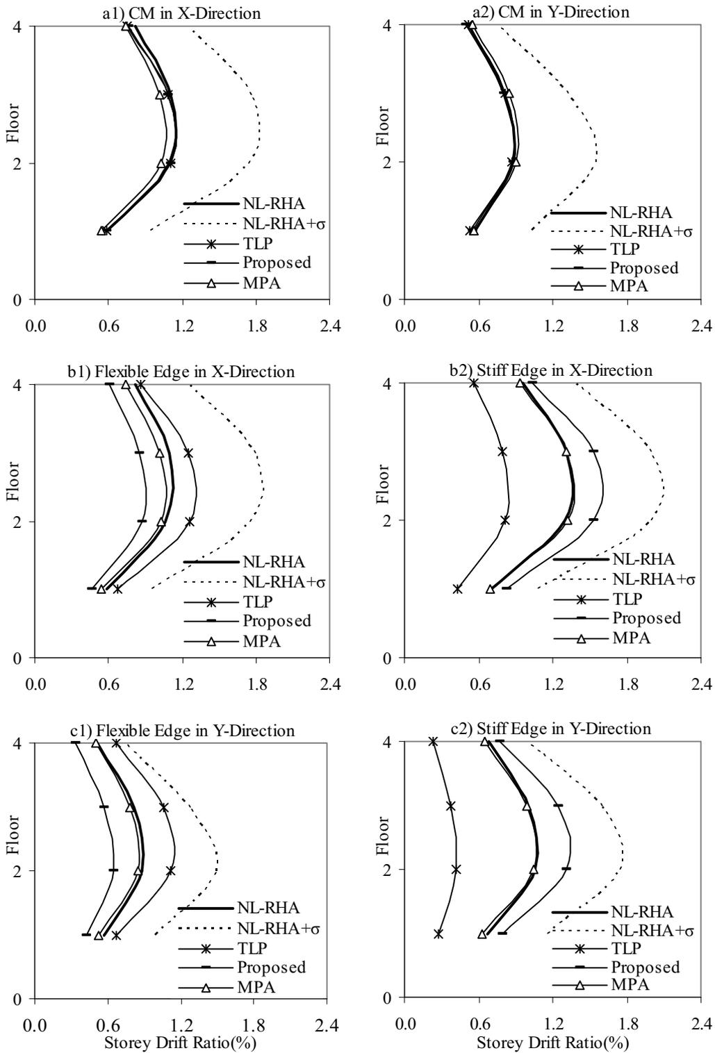
**Fig. 8** Height-wise variation of the storey drifts for the torsionally-flexible 4-storey building: a) at the CM; b) at the flexible and stiff edges in X-direction; and c) at the flexible and stiff edges in Y-direction
