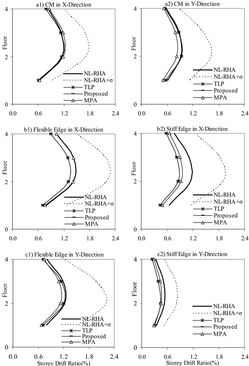
**Fig. 4** Height-wise variation of the storey drifts for the torsionally-stiff 4-storey building: a) at the CM; b) at the flexible and stiff edges in X-direction; and c) at the flexible and stiff edges in Y-direction
