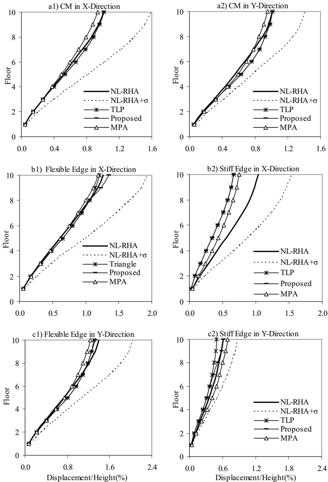
**Fig. 3** Height-wise variation of the displacements for the torsionally-stiff 10-storey building: a) at the CM; b) at the flexible and stiff edges in X-direction; and c) at the flexible and stiff edges in Y-direction
