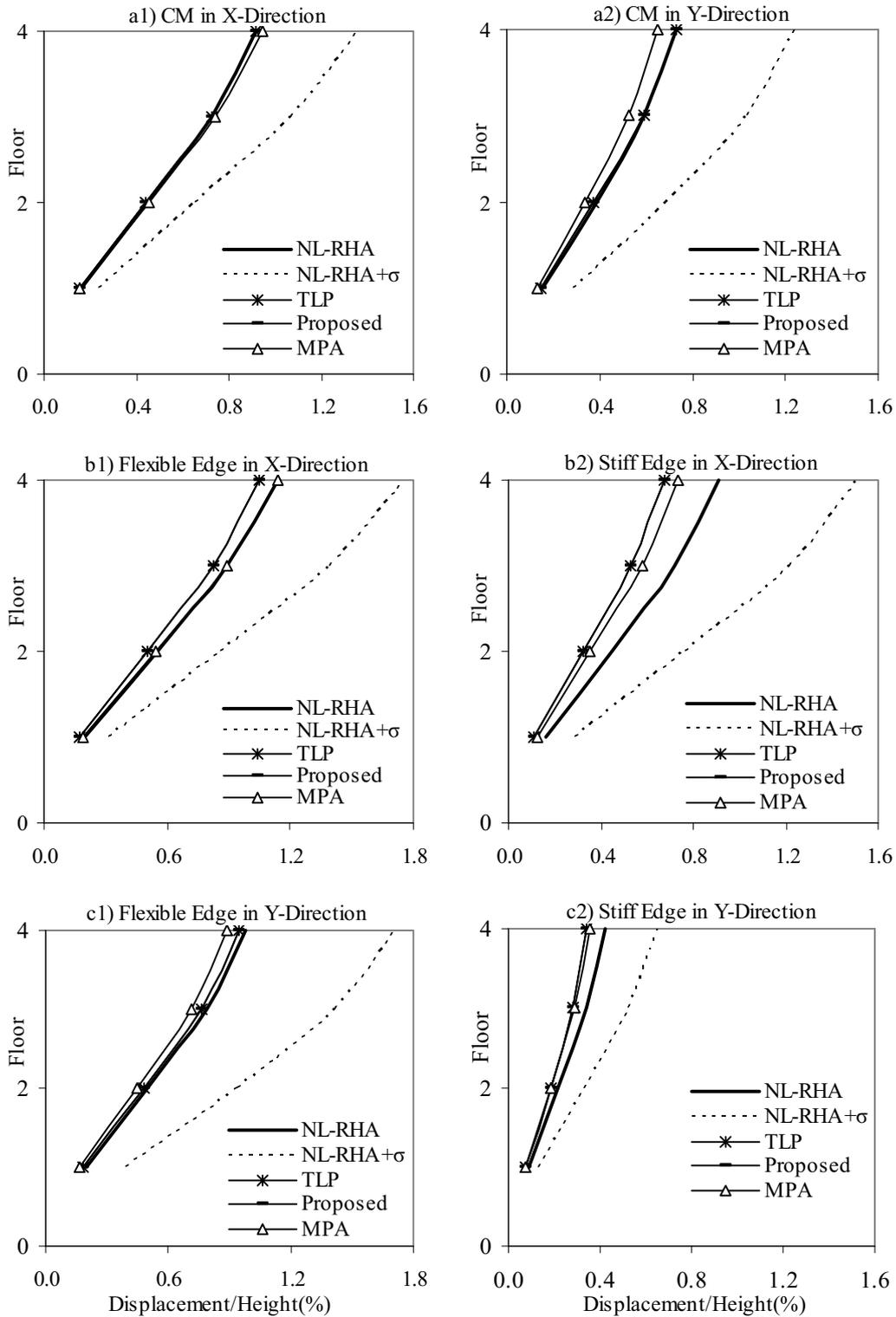
**Fig. 2** (a) Height-wise variation of the displacements for the torsionally-stiff 4-storey building: a) at the CM in X and Y-directions; b) at flexible and stiff edges in X-direction; and c) at the flexible and stiff edges in Y-direction
