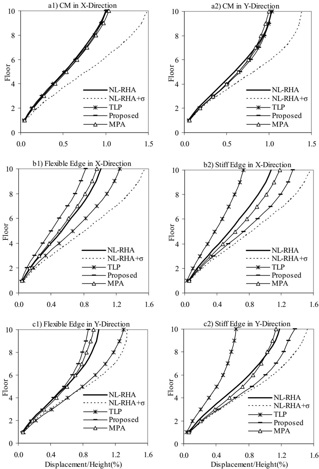
**Fig. 7** Height-wise variation of the displacements for the torsionally-flexible 10-storey building: a) at the CM; b) at the flexible and stiff edges in X-direction; and c) at the flexible and stiff edges in Y-direction
