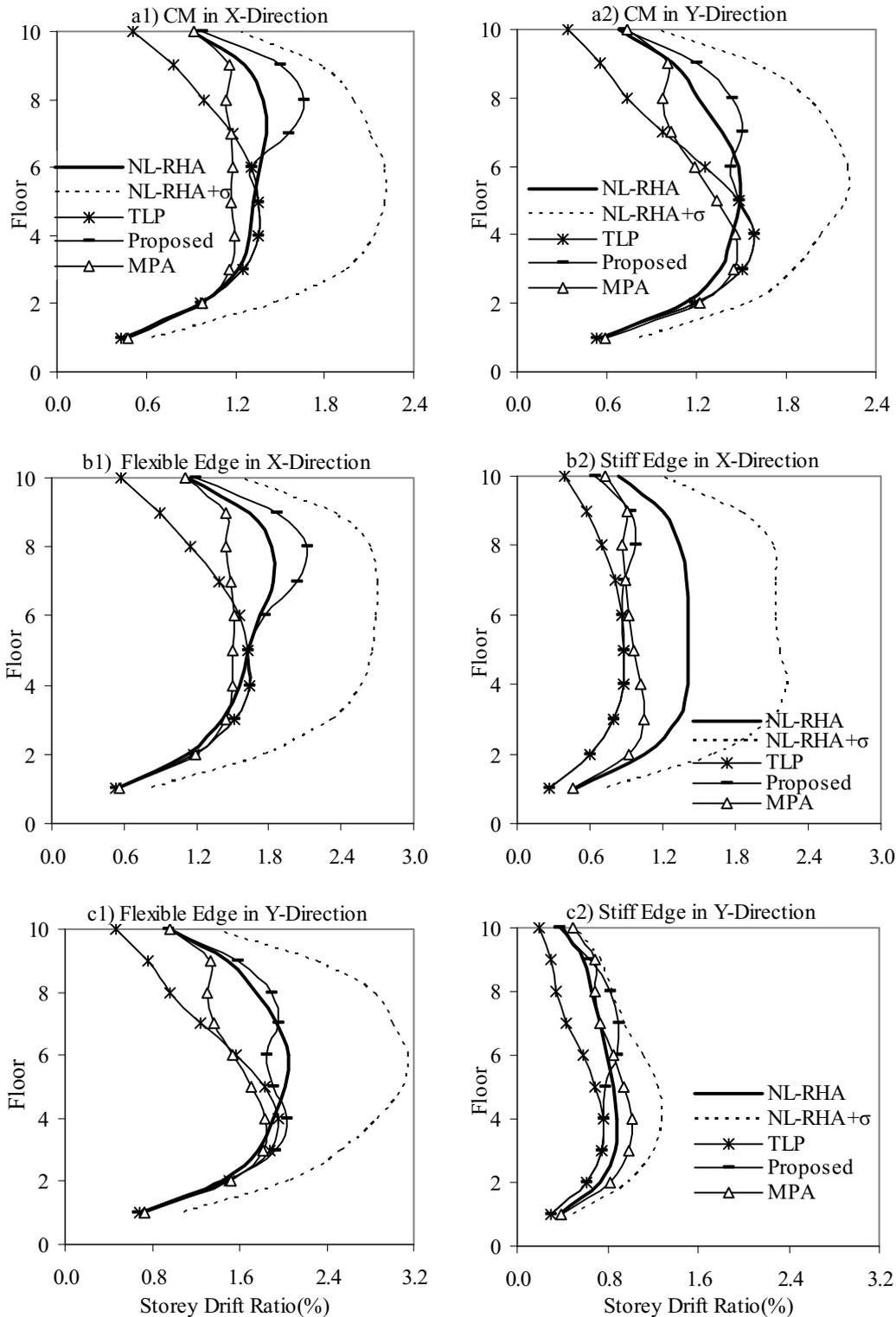
**Fig. 5** Height-wise variation of the storey drifts for the torsionally-stiff 10-storey building: a) at the CM; b) at the flexible and stiff edges in X-direction; and c) at the flexible and stiff edges in Y-direction
