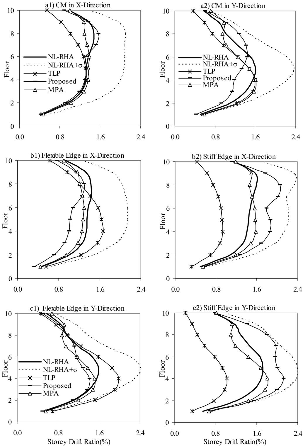
**Fig. 9** Height-wise variation of the storey drift ratios for the torsionally-flexible 10-storey building: a) at the CM; b) at the flexible and stiff edges in X-direction; and c) at the flexible and stiff edges in Y-direction
