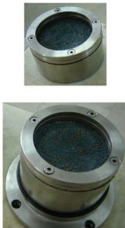
Fig. 3 Modified pedestal and top cap for cemented samples
