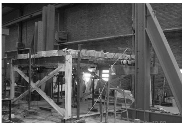
(a) Test set-up and instrumentation framing
