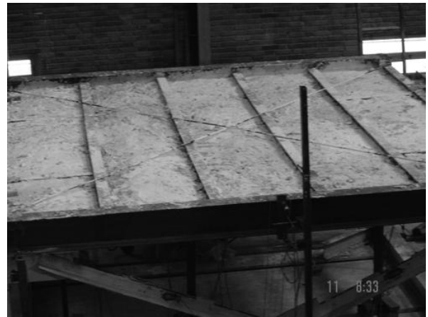
Fig. 9 Specimen-3 retrofitted by single x-bracing diagonal rebar based on FEMA 356 and Iranian standard No. 2800.
