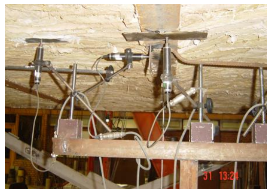
Fig. 7 LVDTs for capturing displacements of the diaphragm in different directions
