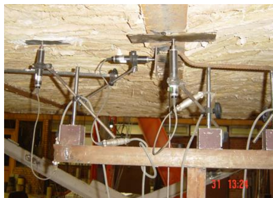
Fig. 7 LVDTs for capturing displacements of the diaphragm in different directions
