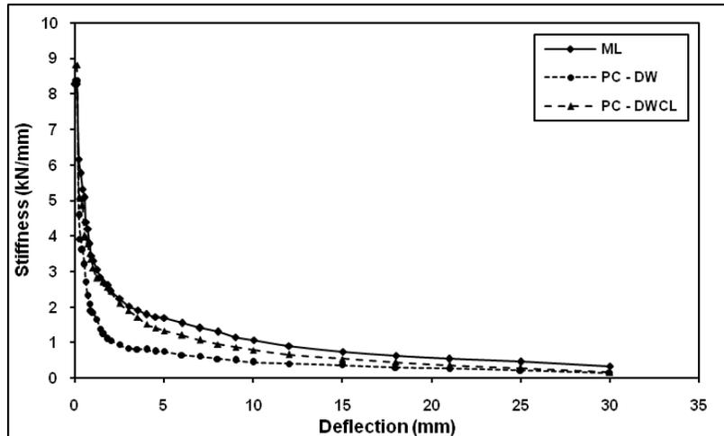
Fig. 13 Stiffness Degradation of three specimens
