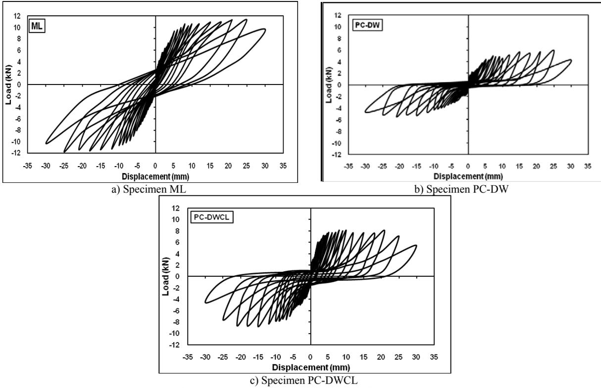
**Fig. 8** Hysteresis Load- Displacement curves of all the specimens
