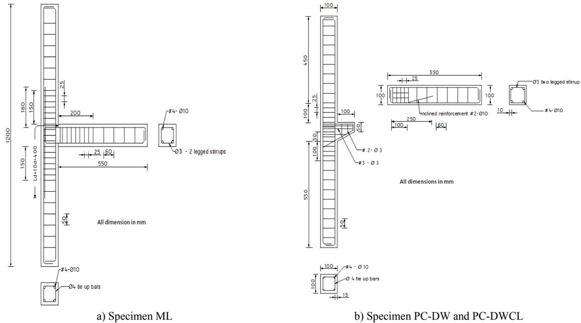
Fig. 2 Reinforcement detailing of specimen PC-DW and PC-DWCL
