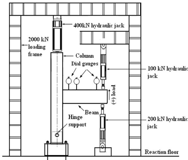
Fig. 4 Schematic Experimental Test Setup
