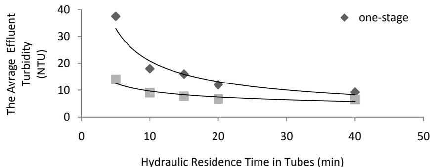
**Fig. 7** The relationship between hydraulic residence time and the average effluent turbidity
