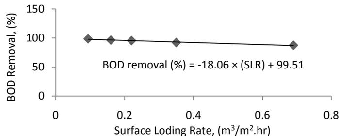
Fig. 10 The relationship between the percentage of BOD removal and SLR
