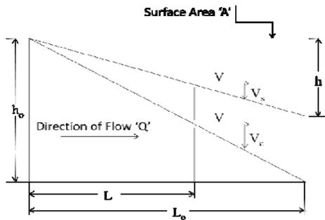
Fig. 1 Ideal settling paths of discrete particles in a horizontal flow basin
