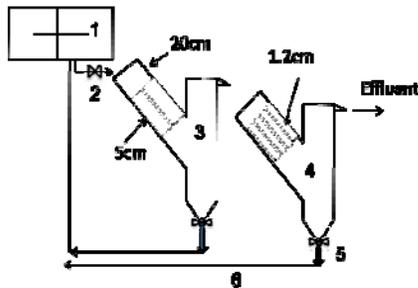
**Fig. 3** Experimental set-up of the two-stage tube settler. (1) Aeration basin, (2) Manual valve to control feed to inclined tube settlers, (3) first stage, (4) second stage, (5) Value to remove settled sludge, (6) return sludge line into aeration basin
