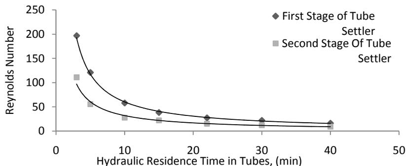
**Fig. 4** The relationship between the Reynolds number and hydraulic residence time, kinematic viscosity of water is  $0.864 \times 10^{-6}$  m<sup>2</sup>/s at 27°C [9]
