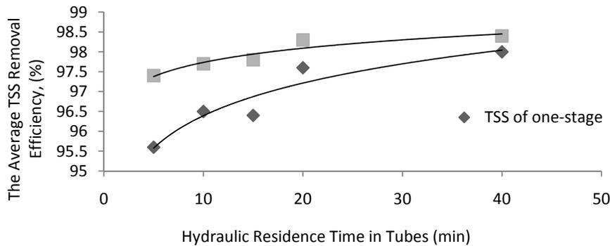
**Fig. 6** The effect of HRT on efficiency of total suspended solid removal.
