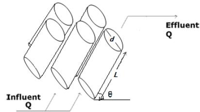
Fig. 2 Schematic of inclined tubes.
