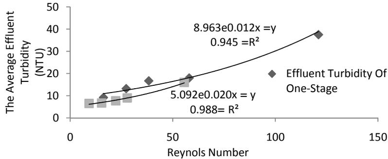
Fig. 8 The relationship between the average effluent turbidity and Reynolds number
