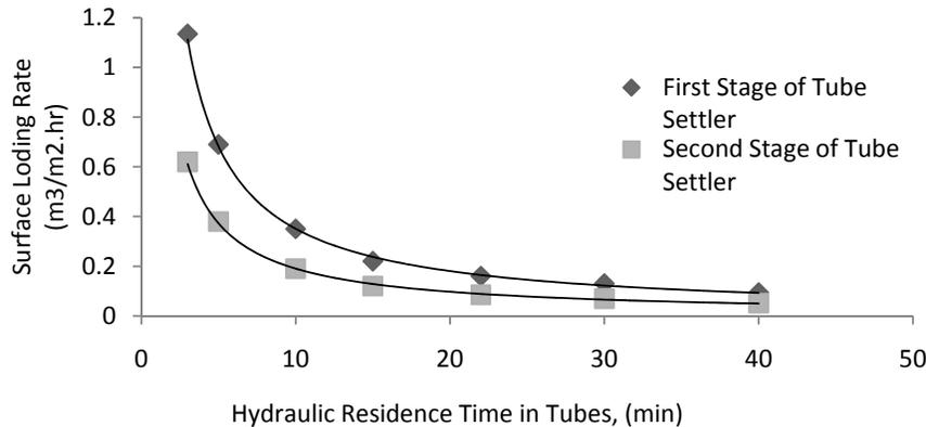
Fig. 5 The relationship between surface loading rate and hydraulic residence time
