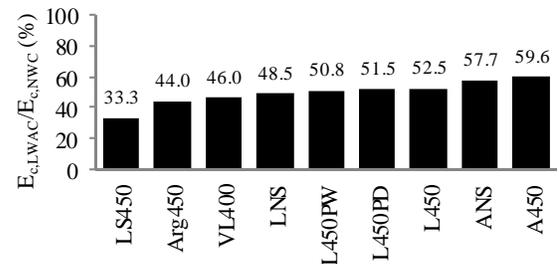
**Fig. 1** Modulus of elasticity of LWAC,  $E_{c,LWAC}$ , in relation to that of NWC of the same composition,  $E_{c,NWC}$
