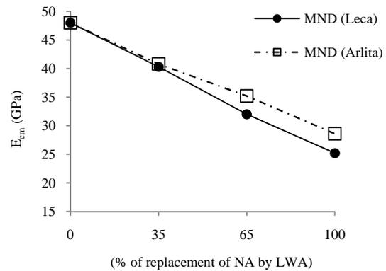
**Fig. 7** Modulus of elasticity at 28 days for different replacement percentages of coarse normal density aggregate by lightweight aggregate
