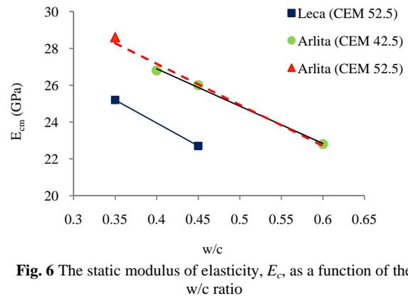
**Fig. 6** The static modulus of elasticity,  $E_c$ , as a function of the w/c ratio
