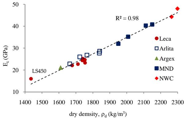
**Fig. 9** Relation between the static modulus of elasticity,  $E_c$ , and dry density,  $\rho_d$
