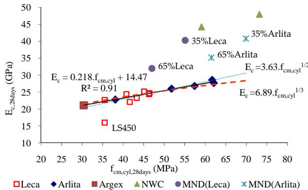
**Fig. 2** Relation between modulus of elasticity,  $E_c$ , and compressive strength,  $f_c$ , at 28 days
