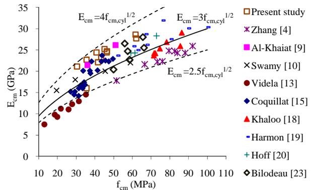
**Fig. 3** Relation between the elastic modulus,  $E_{cm}$ , and compressive strength,  $f_c$ , (different references)
