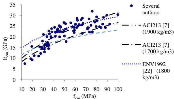
**Fig. 5** Comparison between the experimental results from several authors (including the results of the present study) and those estimated by the main normative expressions
