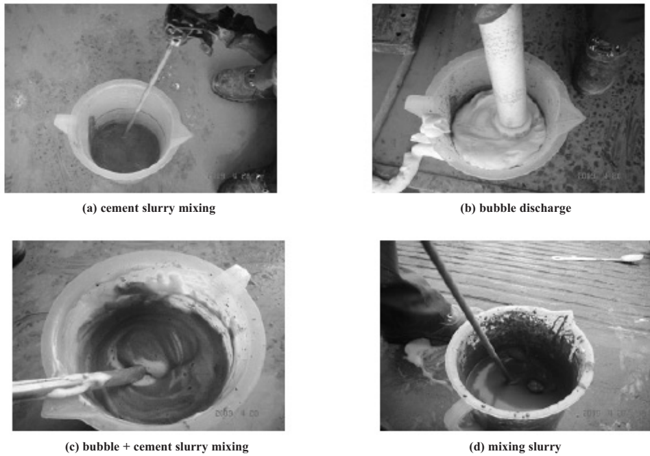
Fig. 3 Lightweight ATS production process
