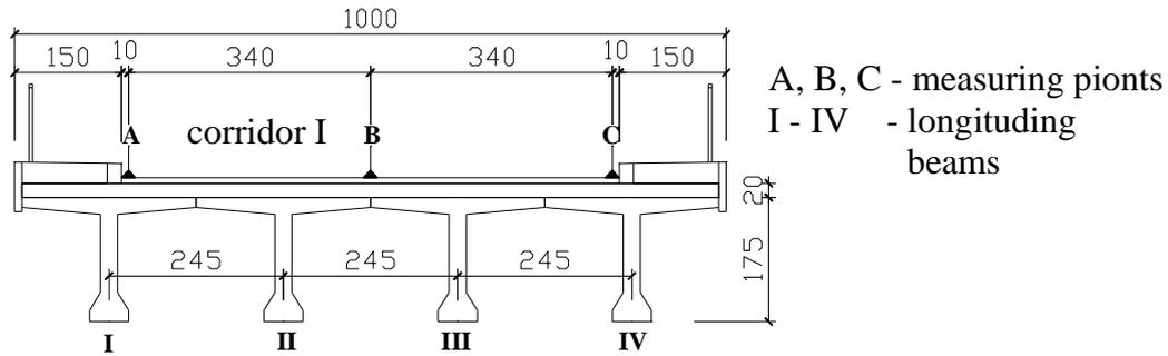
Fig. 4 The Brod bridge cross-section
