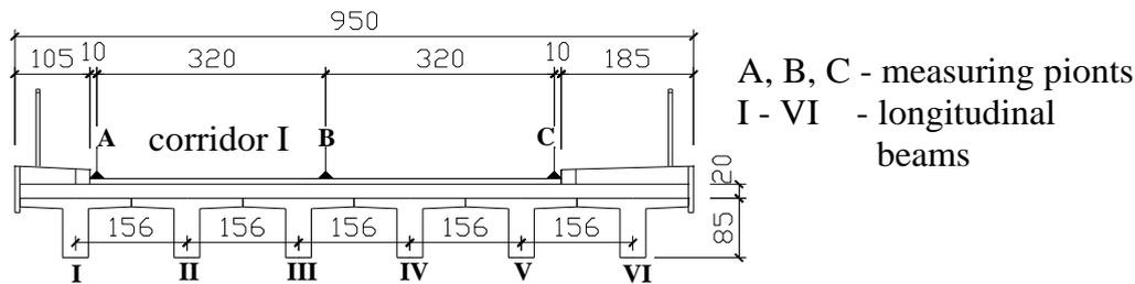
**Fig. 3** The Vinično bridge cross-section
