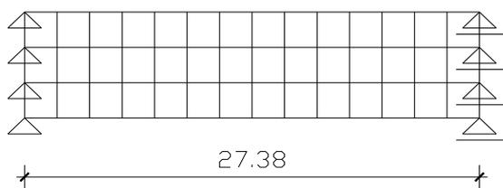
**Fig. 6** The numerical model of the Jamnica bridge
