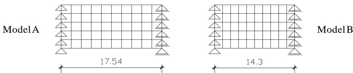
**Fig. 8** The numerical models of the Vinično bridge
