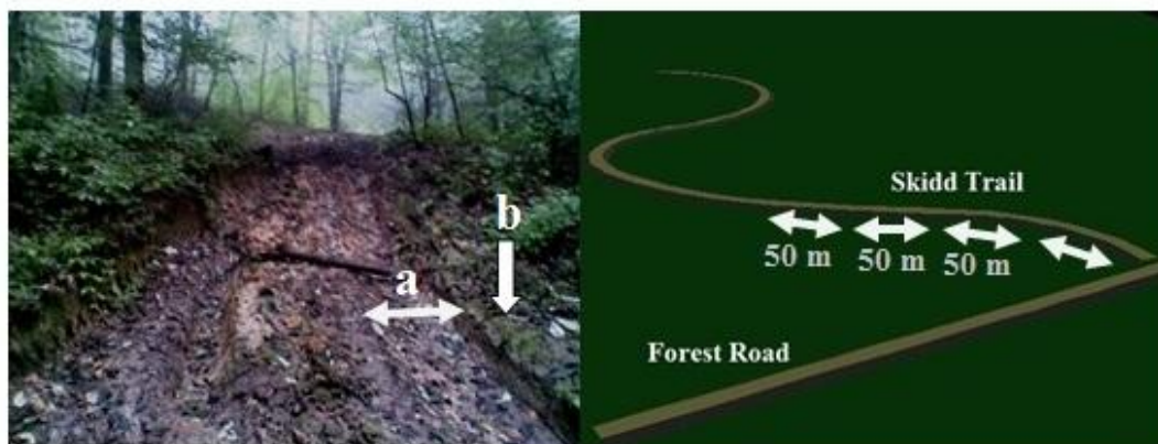
Fig. 2 Sampling for soil measurements; a: Disturbed; b: Undisturbed
