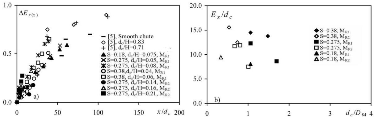
Fig. 4 (a) Rate of energy dissipation over ramp length for base material configurations  $M_{R1}$  and  $M_{R2}$  and comparison with [5] data for  $S=0.07$ ; (b) dimensionless residual energy at the end of the sloping channels
