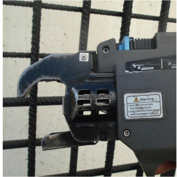
Fig. 4 Close-up of the adjustable pick
