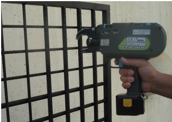
Fig. 6 Battery powered rebar tier
