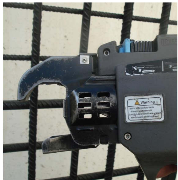
Fig. 4 Close-up of the adjustable pick
