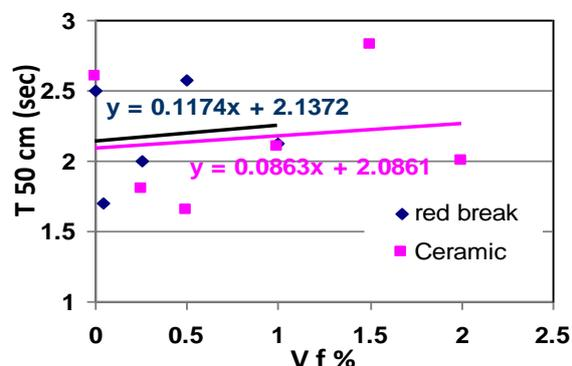
**Fig. 8** Effect of the Steel Fiber Volume Fraction of the Flow Time (T<sub>50cm</sub>)
