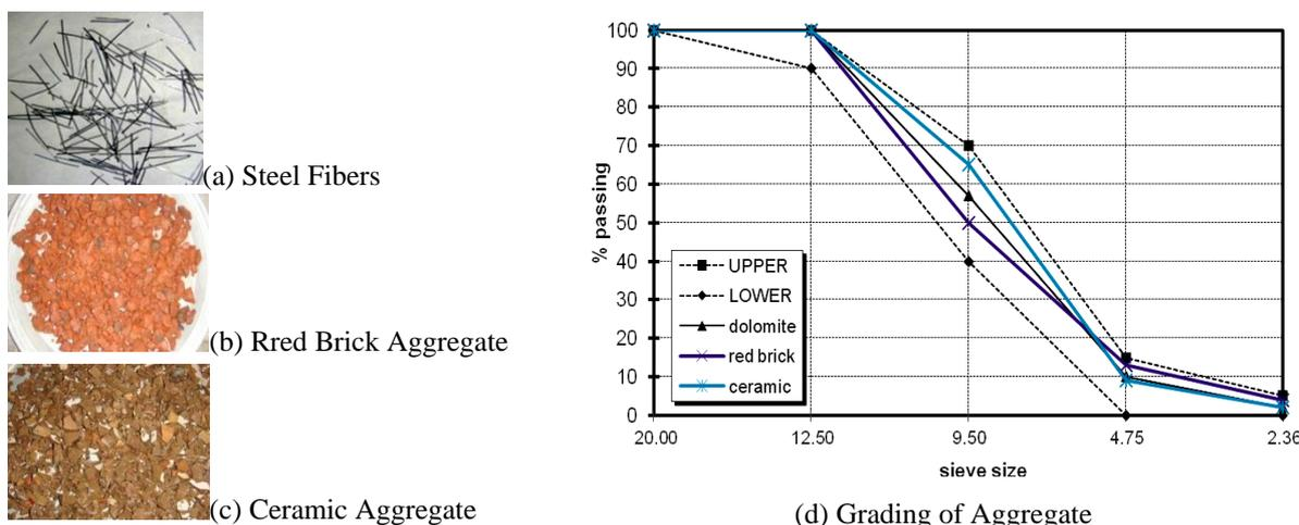
**Fig. 1** Recycled Materials as a Coarse Aggregate
