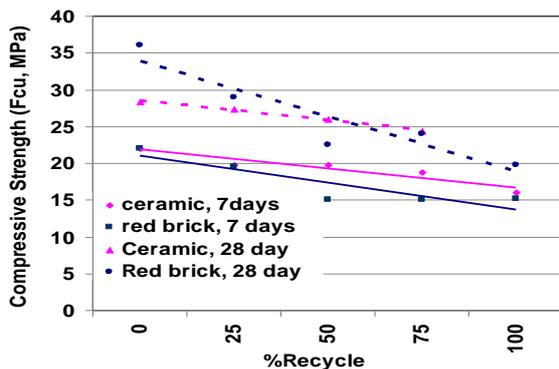
Fig. 5 Compressive Strength for Recycled Self-Compacting Concrete
