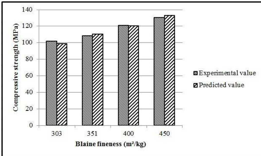
**Fig. 4** Comparison of experimental 270-day compressive strength with predicted 270-day compressive strength for Blaine finenesses of 303, 351, 400, and 450 m<sup>2</sup>/kg
