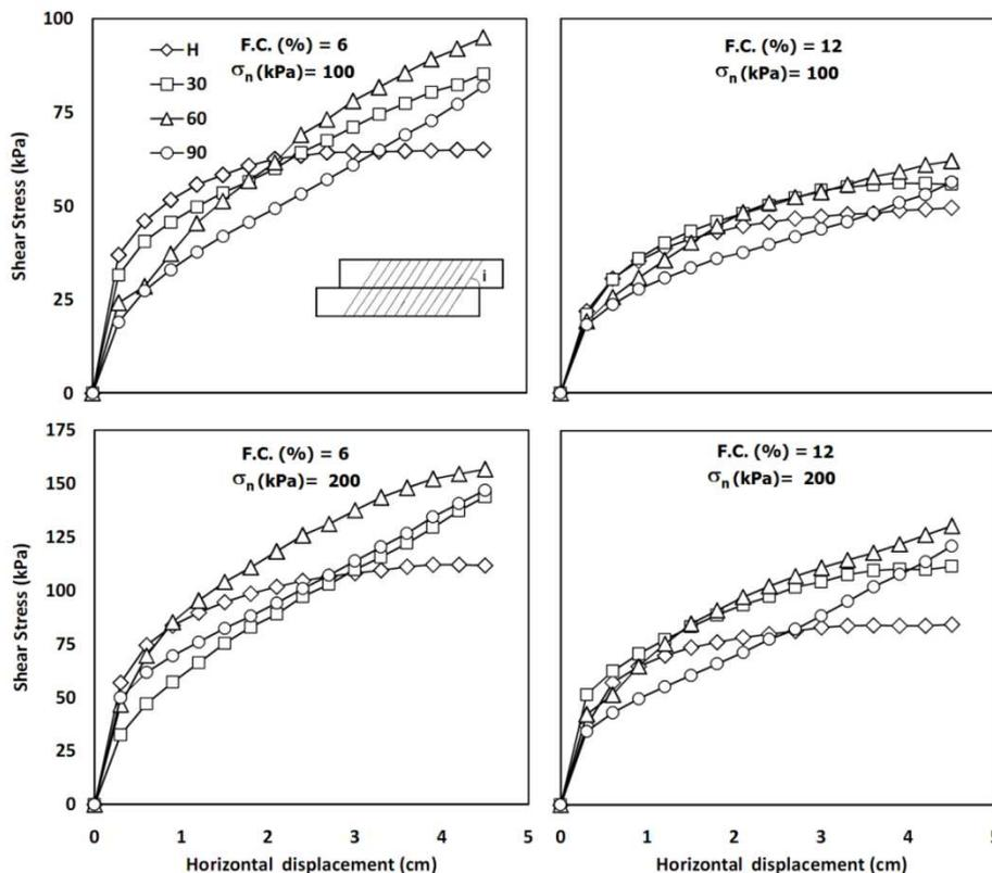
**Fig. 8** Results of tests on MSW samples with different fiber orientation, for fiber contents of 6 and 12% and in two normal stresses of 100 and 200 kPa
