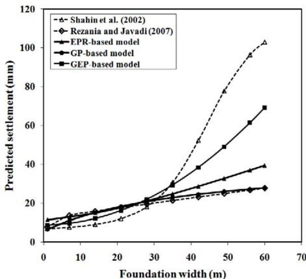
**Fig. 5** Results of parametric study: effect of foundation width
