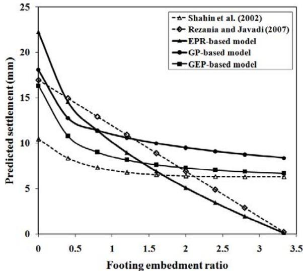
Fig. 9 Results of parametric study: effect of foundation embedment ratio
