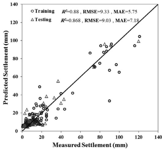
Fig. 3 Comparison of settlements measured and predicted by the GP-based model
