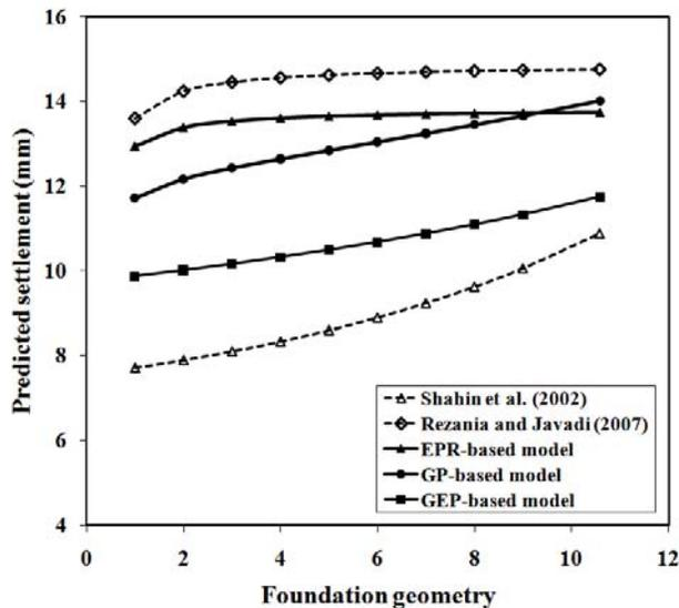
Fig. 8 Results of parametric study: effect of foundation geometry (the ratio of length to width, L/B)
