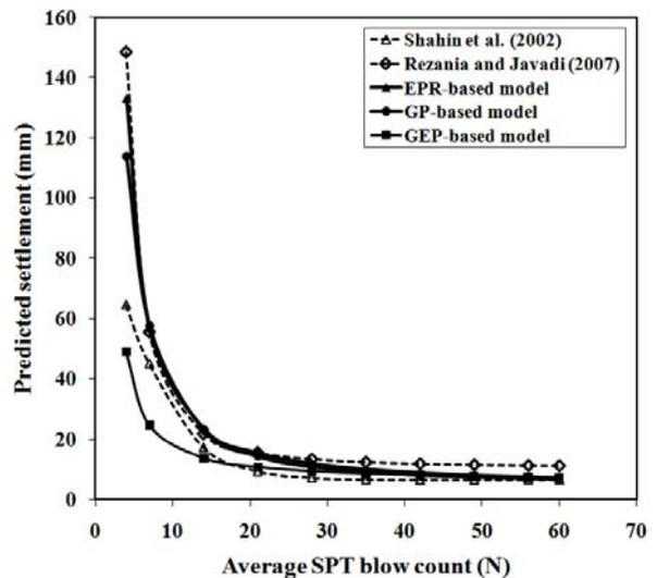
**Fig. 7** Results of parametric study: effect of average SPT blow count
