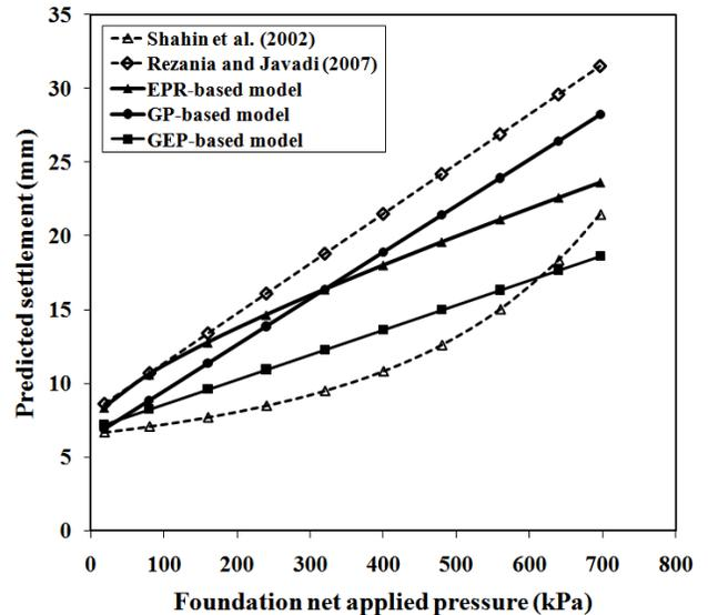
**Fig. 6** Results of parametric study: effect of foundation net applied pressure
