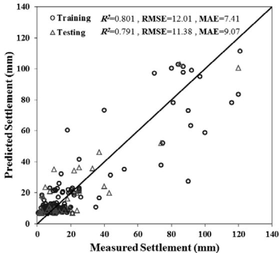
Fig. 4 Comparison of settlements measured and predicted by the GEP-based model
