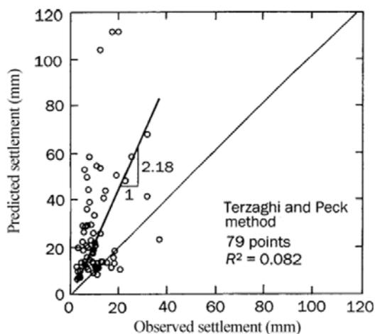
**Fig. 1** Comparison of predicted with observed settlements for 79 foundations based on Terzaghi and Peck method (Sivakugan et al., 1998)
