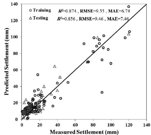
**Fig. 2** Comparison of measured versus predicted settlements obtained from the EPR-based model
