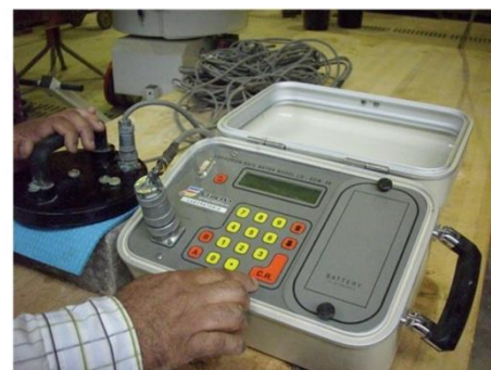
Figure 4 GECOR-8 (Corrosion Measurement device)
