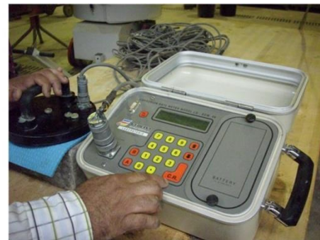
Figure 4 GECOR-8 (Corrosion Measurement device)
