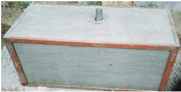
Fig. 2 Rectangular tank filled up by non-cohesive target material
