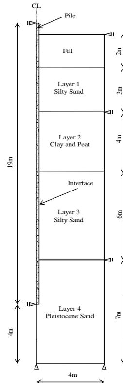
Fig. 4 Axisymmetric pile-soil model for pile driving simulation.
