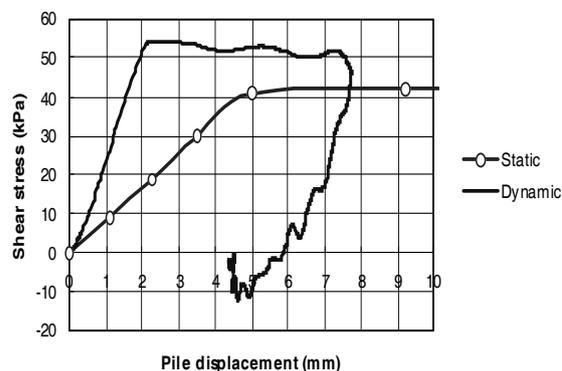
Fig. 9 Static and dynamic shaft response at 6m above tip.
