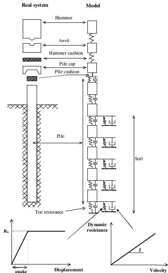
Fig. 1 Pile-soil-hammer system based on Smith model [3].
