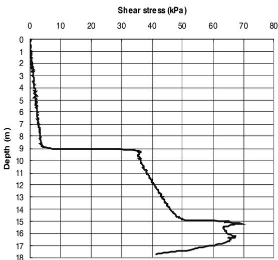
**Fig. 12** Calculated distribution of shear stress on the pile shaft; compares reasonably good with the CPT profile.
