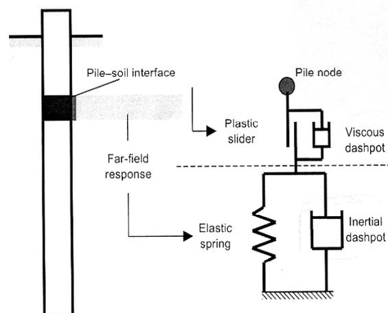
Fig. 2 Dynamic soil-pile shaft model to account for inertial damping [1].
