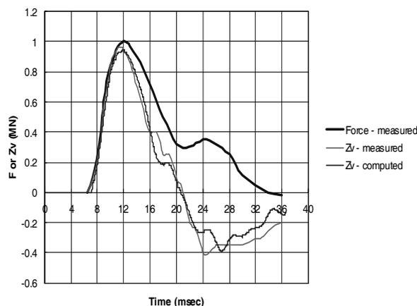
Fig. 6 Measured force, and measured and computed  $Z_v$  wave traces.
