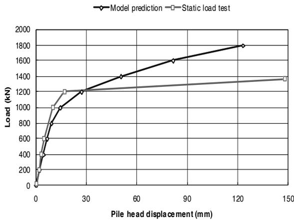
**Fig. 11** Static load test simulation result compared with the real test result.
