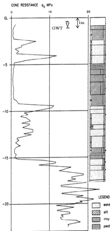
Fig. 3 Soil profile and CPT results [16].
