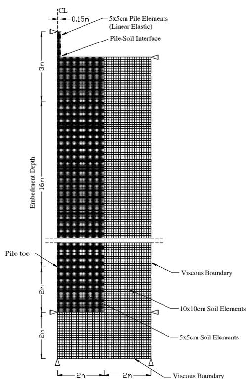
**Fig. 5** Finite difference mesh for the axisymmetric pile-soil model.
