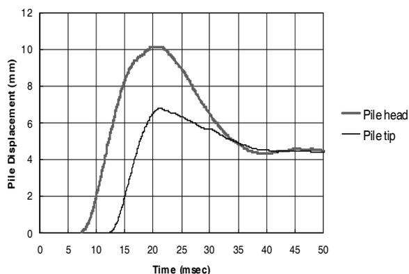
Fig. 8 Pile head and tip displacements versus time.
