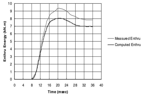
**Fig. 7** Measured and computed applied energy (Enthru) versus time.
