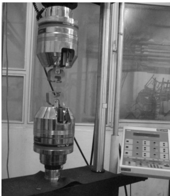
Fig. 5 Experimental setup for BRB tests
