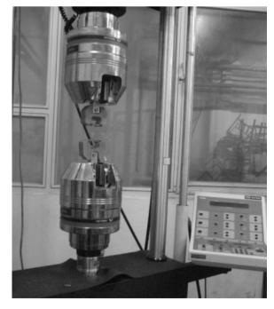
Fig. 5 Experimental setup for BRB tests
