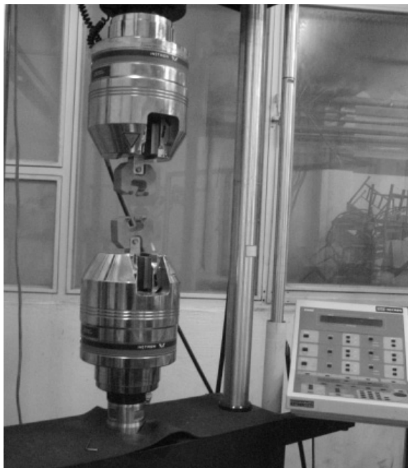
Fig. 5 Experimental setup for BRB tests
